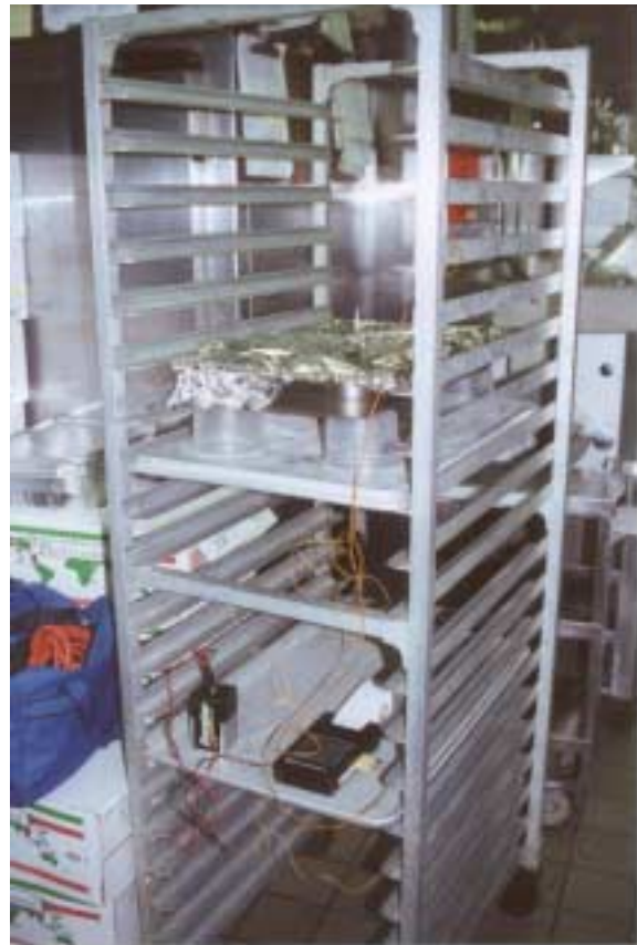
Figure 4. Rack with no fan set up for pan cooling
