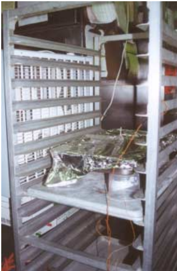
Figure 3. Rack with fan and 2" pan for cooling
