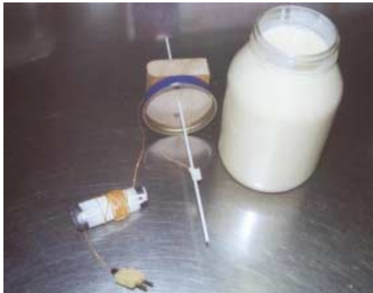
Figure 2. Picture of thermocouple placement in 1-quart mayonnaise jar
