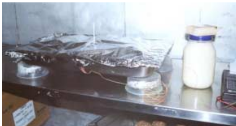
Figure 3. Picture of Alfredo Cream Sauce cooling 1" deep in a 12"x20"x2-1/2" stainless steel pan and in 1-quart mayonnaise jar
