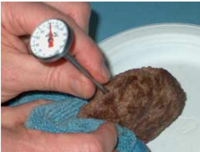
**Figure 4. Measuring temperature of a ¼-lb. hamburger, hand-molded with ground beef purchased at grocery store, with bimetallic coil thermometer**
