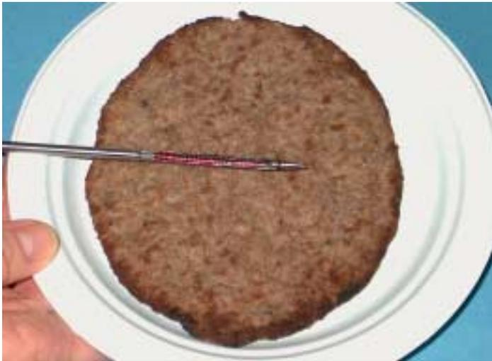
**Figure 2. Cut-away of bimetallic coil thermometer and ¼-pounder from fast-food chain**
