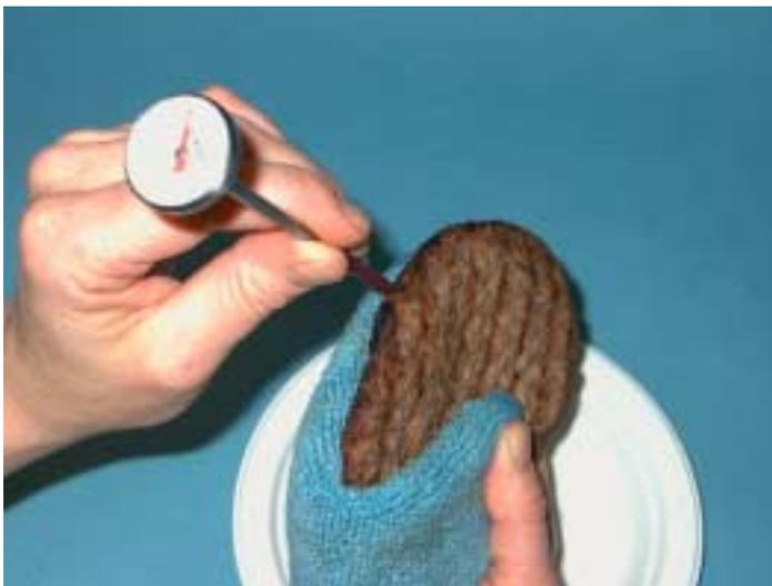
**Figure 3. Trying to insert a bimetallic coil thermometer into the edge of a ¼-pounder from fast-food chain**
