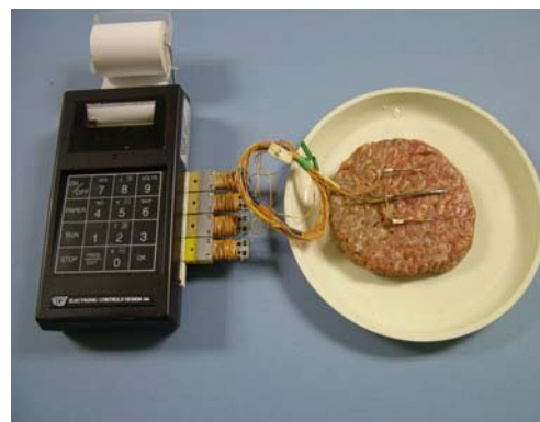
Figure 2. Data Logger with Three-pronged Temperature-measuring Device
