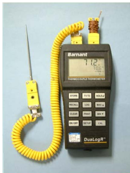
Figure 4. Thermocouple with thin-tipped, 0.040 probe
