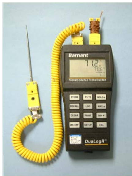
Figure 4. Thermocouple with thin-tipped, 0.040 probe
