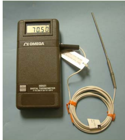
Figure 7. Omega HH1 thermistor thermometer
