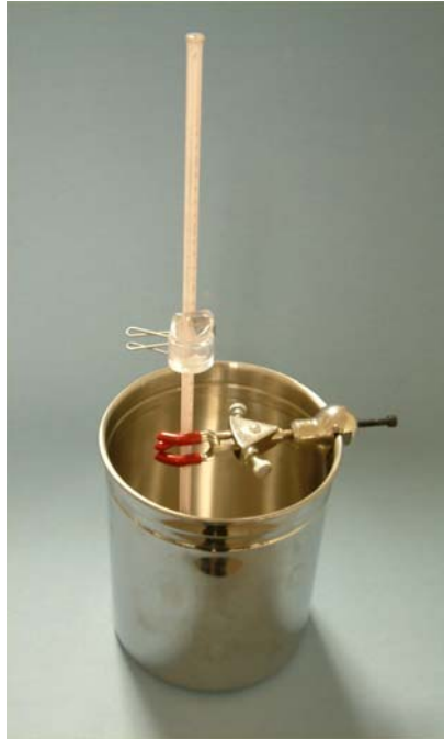
Figure 5. Glass thermometer for calibration in boiling water
