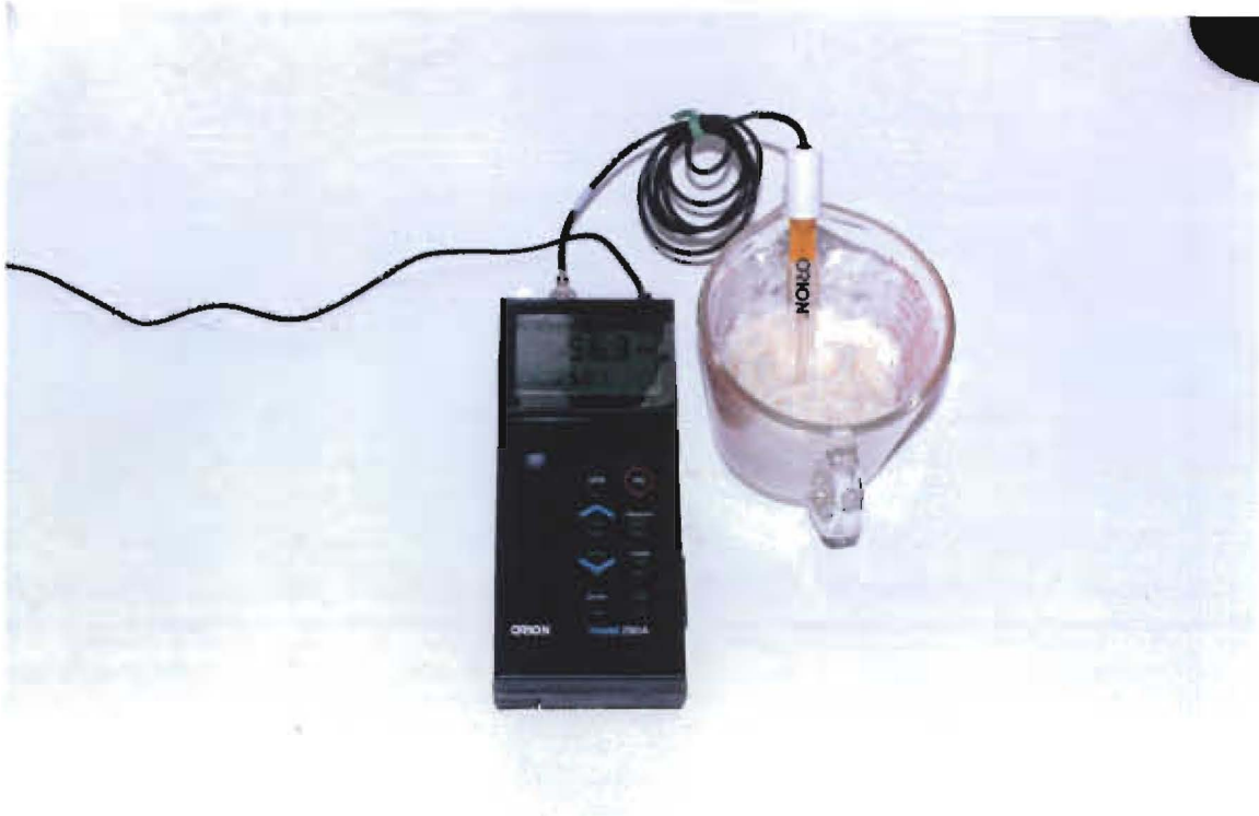
Figure 1 Hungry Jack Instant Mashed Potatoes Orion E_h electrode mv = +56.3 ~1/4 inch below the food surface
